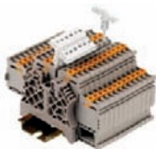
This tag holder is specially conceived for the IDK 1.5N two-tier terminal of the I-series. The flexible hinge mechanism allows cross-connections to be connected or disconnected at little effort. It can be fitted with four DEK 5 tags or two WS 10/5 Middle connector markers.
