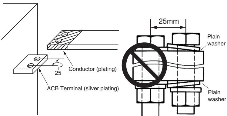
Since fault current flowing through the conductors cause large electromagnetic forces, the conductors should be secured firmly, using the values in the below table as a reference. Max distance between fixing support and ACB bus bar should be less than 200mm.
