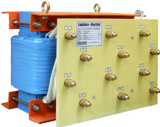
Auto starter transformers is applicable to AC 50Hz three-phase squirrel cage induction motor with rated voltage of 380V, rated output capacity of 450kW and below for reduced-voltage starting under intermittent duty. It makes use of voltage reduction feature of the transformer to reduce motor starting current so as to relief influence of motor starting current on power transmission network
