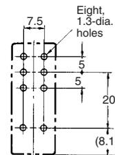
**Mounting Height of Relay with Back-connecting Sockets**
