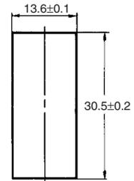
Recommended thickness of the panel is 1.6 to 2.0 mm
